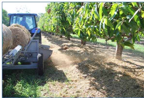
Mulching methods: Side-throw slasher at Blushing Acres and bale buster at Samdara.
