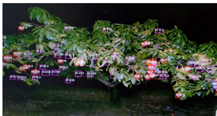
An example of processing of machine vision footage. The software counts fruit using technology similar to facial recognition.
