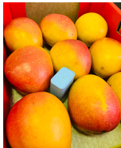
SIM temperature logger in a mango tray.
