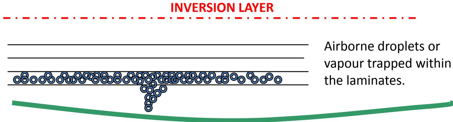
Laminates, only visible due to the small water droplets trapped within them (typically less than 30 microns)
