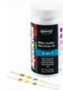
Water quality test strips can be used to assess pH and water hardness in the field.
