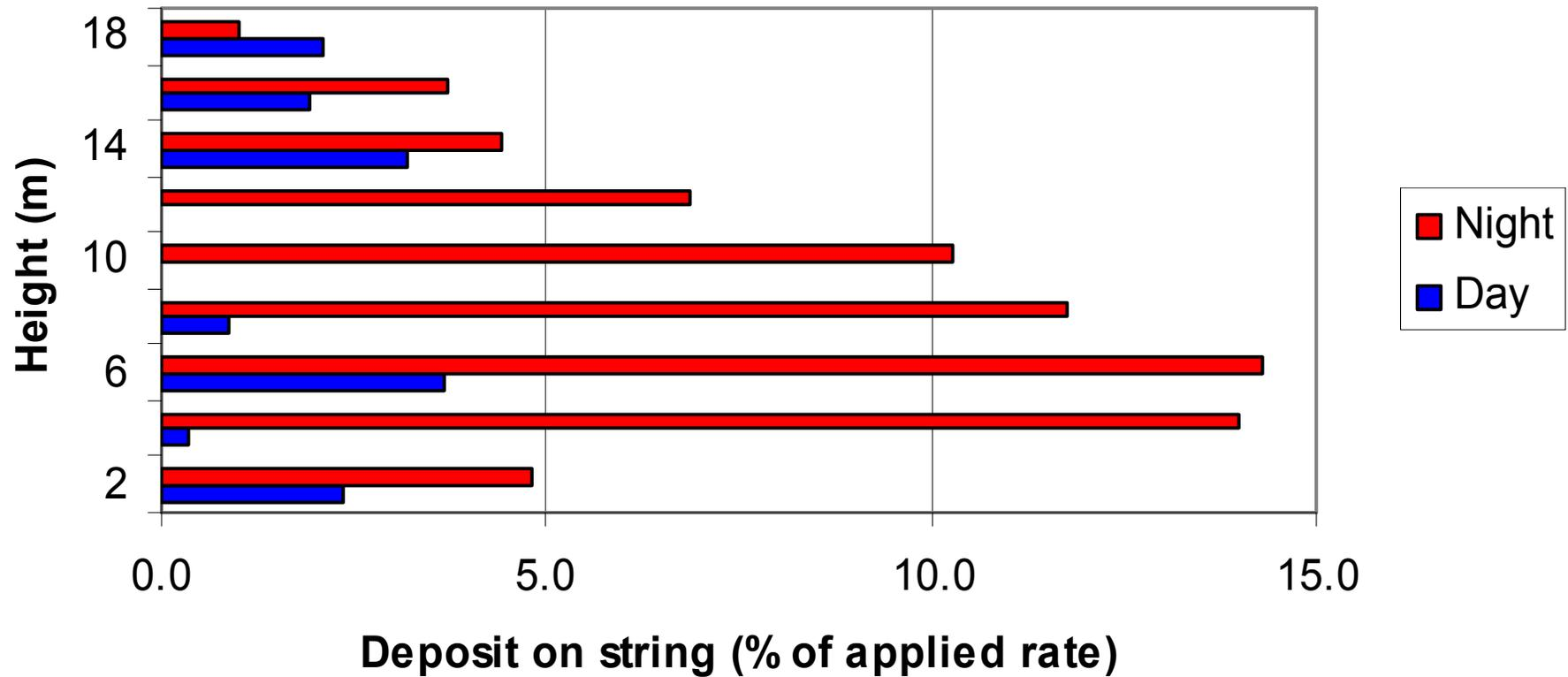
The gentle flow of cold air down minor slopes will intensify low level inversions. The light winds within the inversion may carry chemical droplets far from the target area.
