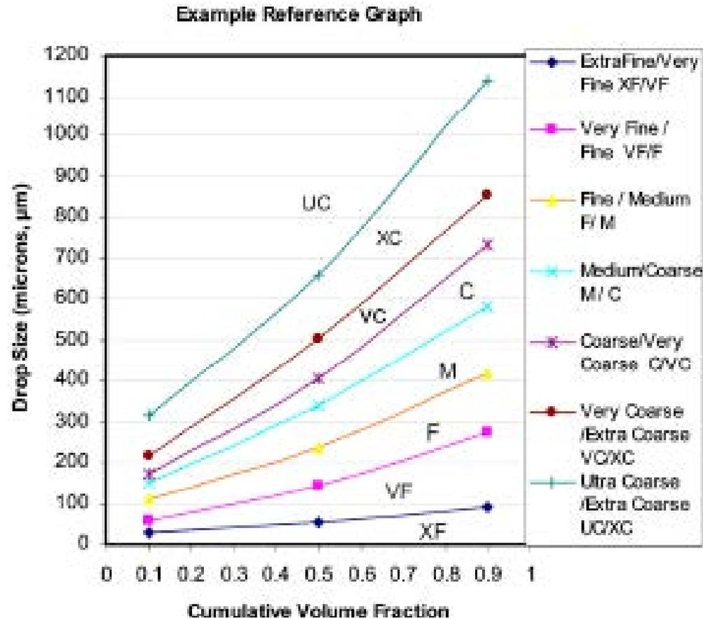
Figure 1 – Sample reference graph developed from measurements averaged from three types of laser instruments. NOTE: To view figure in color please go to <http://www.asabe.org/standards/image/s/s572images.html>
