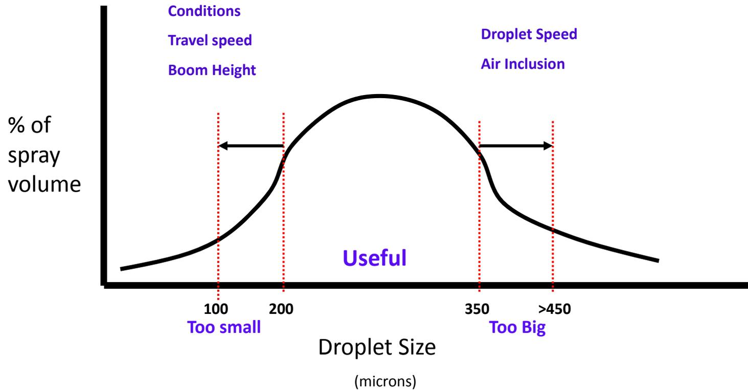
Changing nozzle type shifts the curve, less small droplets, but more big droplets
