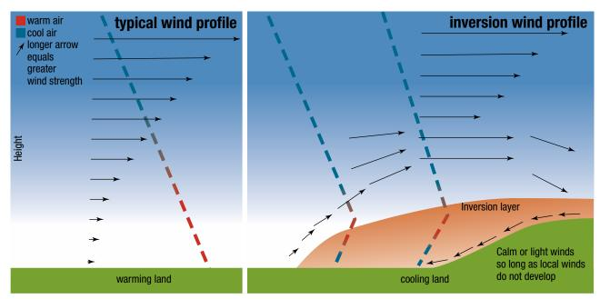
FIGURE 2: Air movement under a surface temperature inversion differs from a typical wind profile (left). Surface winds de-couple from the surface, accelerate and flow over the inversion. Within the inversion, winds are typically light and often drain down slope, regardless of the overlying wind direction. Under an inversion the shape of the landscape also influences the direction in which airborne droplets will move (right).
