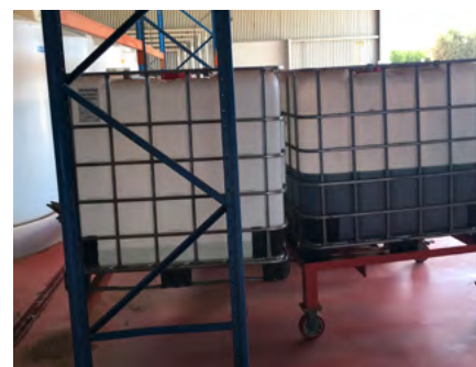
Fertigation mixing and holding tanks: Fertigation systems vary in size depending on your requirements, from the need for large holding tanks (left), to in-field injection points (top right), to the use of 1,000L fertilizer shuttles (bottom right). Photographs provided by AgriHort Solutions.
